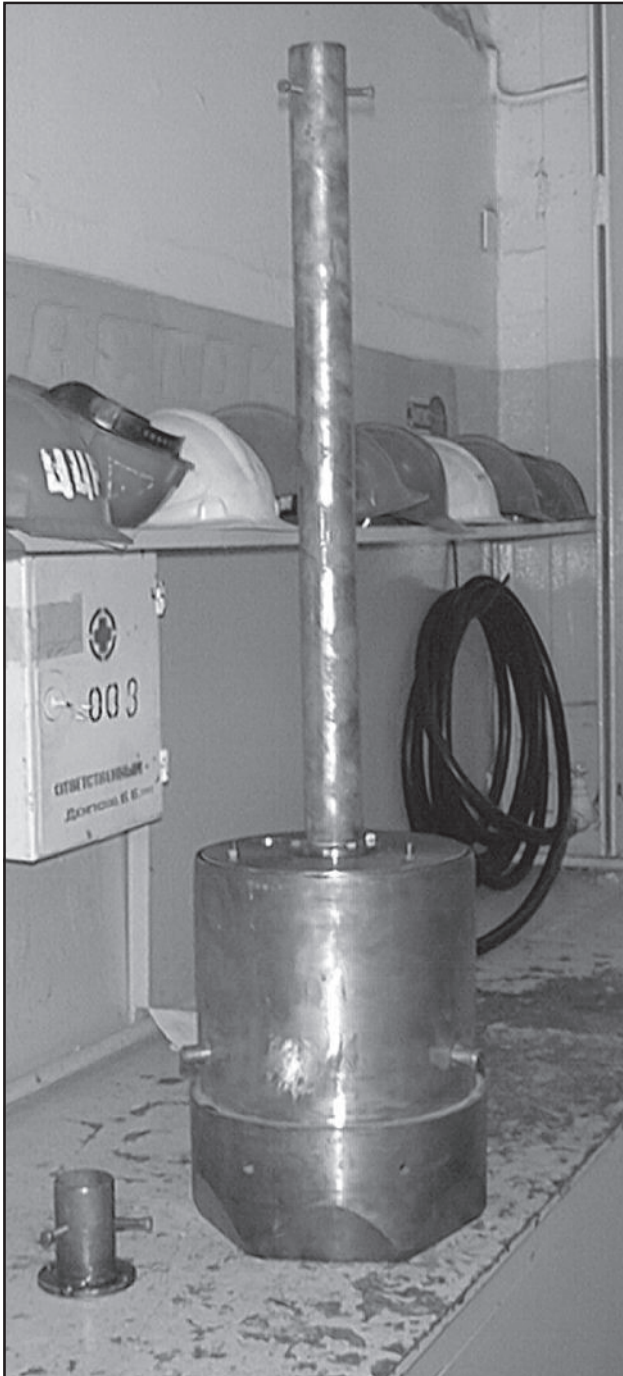
Figure 3. Adapter of the test SFAT device for attachment to the refuelling machine.
