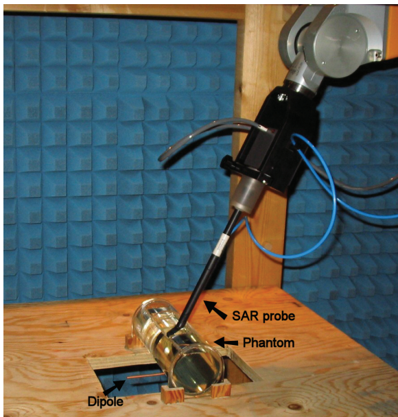
Fig. 7. Phantom setup for validating simulated values of SAR in the skin of human.
