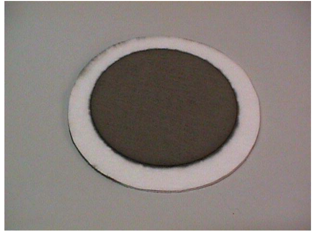
Figure 5. A filter exposed to 5 \text{ mg/cm}^2 of aerosol containing 25 wt-% of diesel fume particles and 75 wt-% of SAE fine dust. Diameter of the darkened area, where the particles are collected, is 15 cm.
