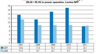
Integrity of primary circuit: Corrosion products; Maximum iron concentration in primary coolant (Fe-tot µg/l) in power operation, Loviisa NPP
