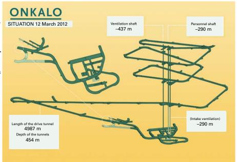
**Figure 2.** Plan of the underground rock characterisation facility (Onkalo) and status of the construction on 12 March 2012 (Posiva Oy).
