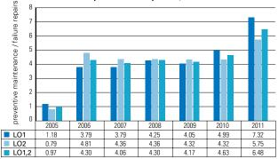
was markedly different from the previous years as concerns the number of fault repairs and amount of preventive maintenance. The number of maintenance operations on OLC equipment reduced from the previous year by 19%, so that the reduction in preventive maintenance operations was 14%, while the reduction in fault repairs was 39%. Due to the fact that the reduction was different in the different types of work, their ratio changed significantly from 4.6 in 2010 to 6.5 in 2011.
