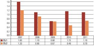
Integrity of primary circuit: Corrosion products; Maximum cobalt-60 activity concentration (kBq/m<sup>3</sup>) in primary coolant related to shutdowns, Olkiluoto NPP
