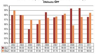
Combined leak rate of containment penetrations and air locks compared to the leak limit, Olkiluoto NPP
