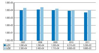
placements exists. The iron content of feedwater is affected by corrosion and the filter material used in the ion exchangers of the condensate purification system. The licensee is investigating the reason for the increase in iron content.
