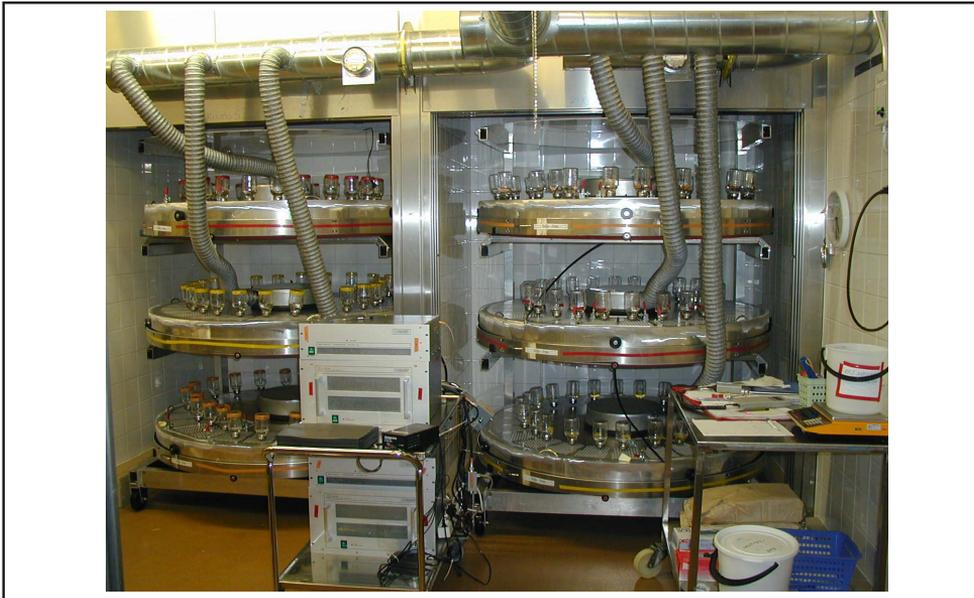
**Figure 1.** Parallel plate chambers for exposing rats to 900 MHz radiofrequency fields. The plastic rat cages are inside the chambers under the drinking vessels. The fresh air for rats is circulated from the tubes in the centre of each chamber. The electromagnetic field is produced with a real GSM-phone and amplified with power amplifiers and controlled with PC; all these in centre of figure.
