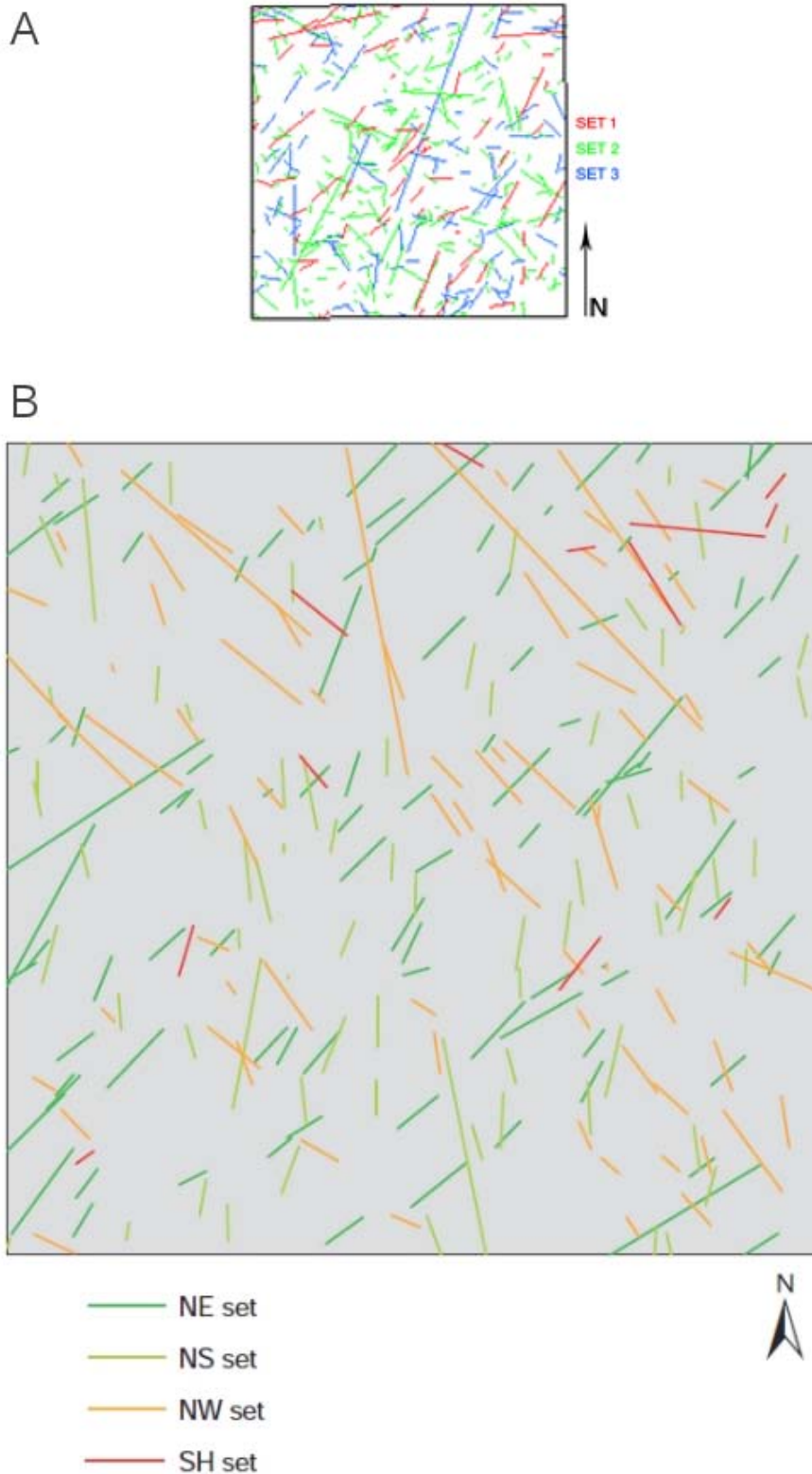
Figure 7. Examples of horizontal cross-sections through simulated fracture populations based on geological DFN models for Olkiluoto and Forsmark. Upper plot shows fracture traces from a simulated 20 m × 20 m fracture trace map representing Olkiluoto outcrop OL-TK11, with colors indicating fracture sets: Set 1 in red is subhorizontal set; Set 2 in green is N-S striking set; Set 3 in blue is E-W striking set (from Tuominen et al., 2006, Figure 6-1). Lower plot shows fracture traces in a simulated plane through a 50 m × 50 m × 50 m cubic volume, based on one alternative DFN model for fracture domain FFM01 at Forsmark, with colors indicating fracture sets as shown in the legend, SH = subhorizontal (from SKB, 2008, Figure 5-40). Note that these simulations represent fracture domains at different depths for the two sites.
