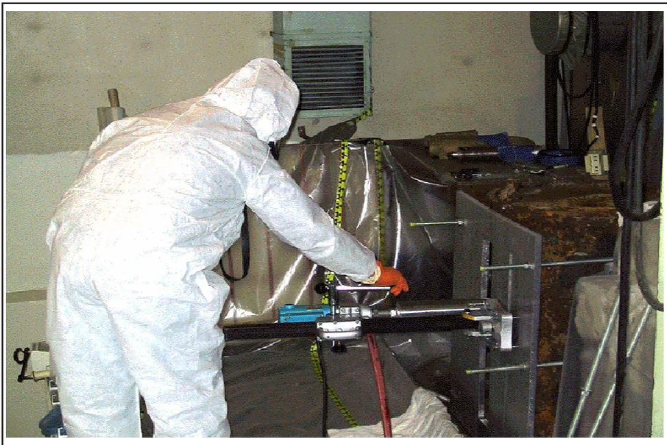
Figure 2. Drilling cores from drum no. 6.
