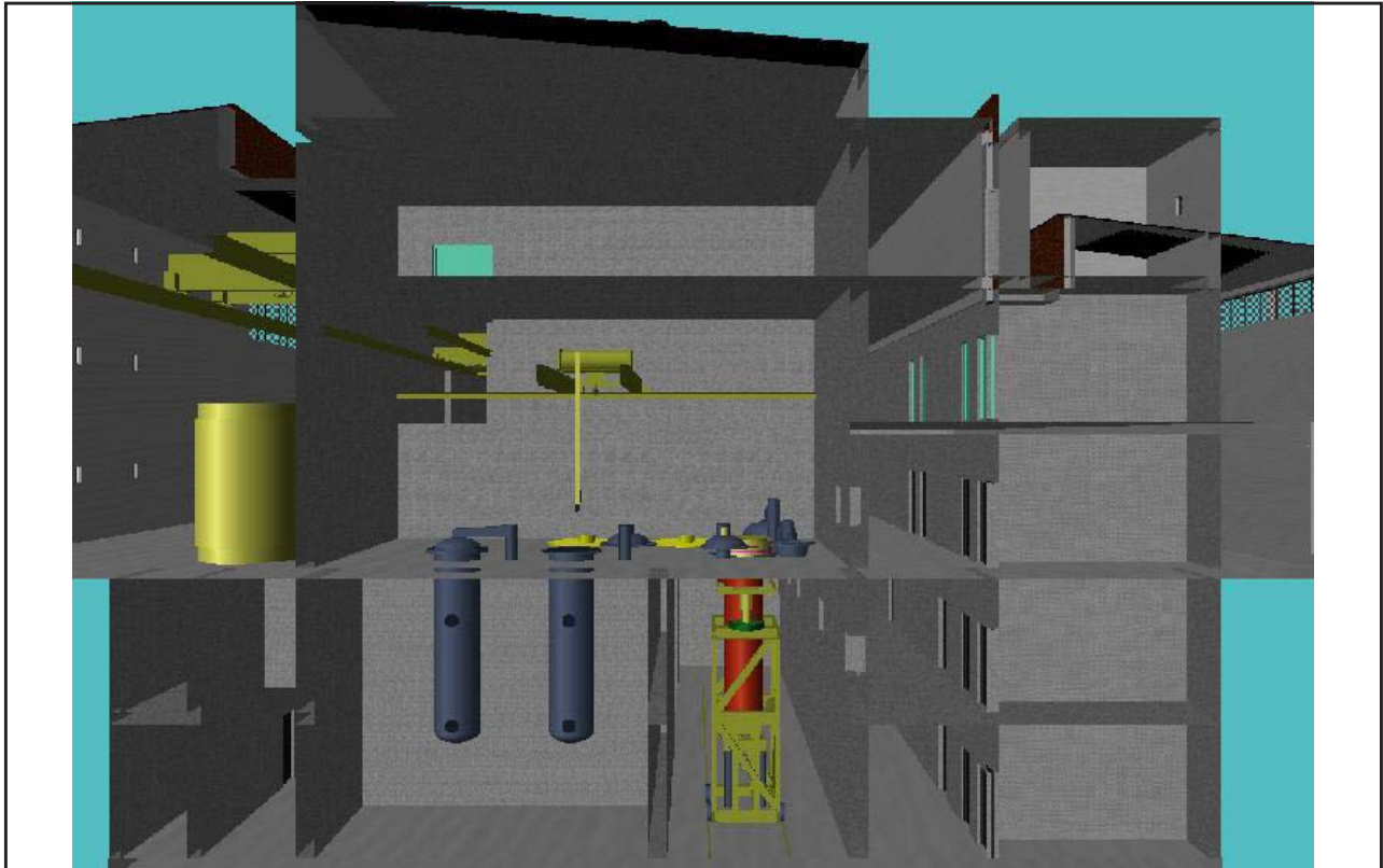
Figure 10. Cross section of the hot cell (1) and adjacent rooms. Two cylinders (2) under the hot cell are reservations for drying autoclaves, buffer positions and/or measurement positions. Cask transport and receiving area is on the left (3) and canister transfer corridor (4) is below the hot cell on the right. A canister shown in the transfer corridor has been docked into its position. Cask docking positions are not shown in this figure.
