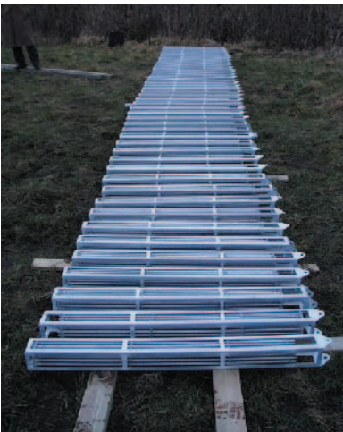
Figure A1-2. Source term used in the December 2000 test. The elements were placed in a row to decrease attenuation. The row was 15 metres long.
