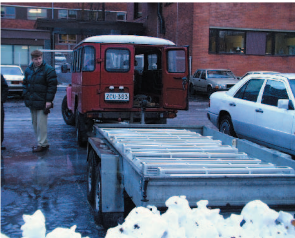
Figure A1-1. Source term used in the December 1999 test. The elements are in two beds.
