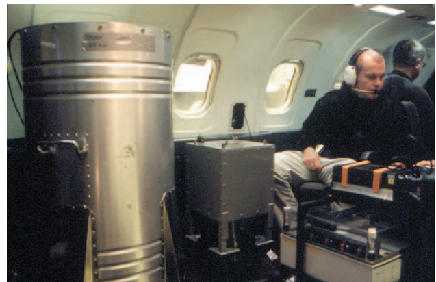
Figure A1-6. The Learjet 35 flying above the target and the installations in the cabin. The large “barrel” at the front is the 6.83 litre (11.5 × 4 inch) NaI detector; the second detector, installed inside the cube, is a 70% HPGe detector and ahead of the operators are spectrometers and a computer.
