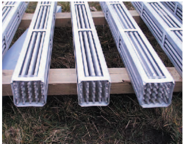
Figure A1-2. Source term used in the December 2000 test. The elements were placed in a row to decrease attenuation. The row was 15 metres long.
