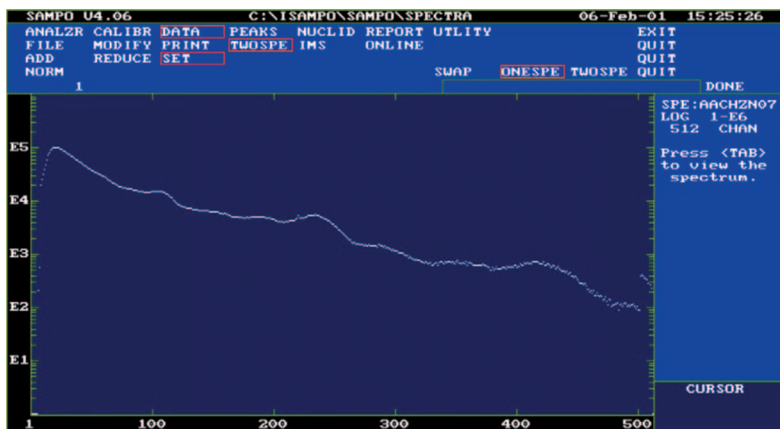
Figure A1-8. Sum spectra of all the spectra recorded with the large NaI (11.5 × 4 inch, 6.83 litres) detector in the 2000 exercise. Clear broadening of the spectra can be detected.
