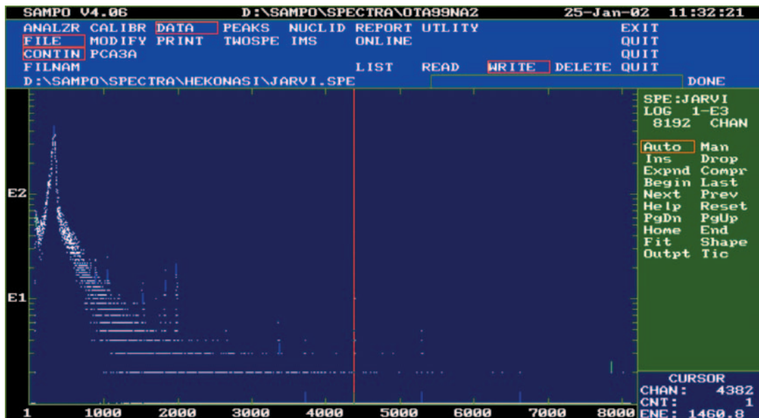
Figure A3-3. Background spectra 100 metres above lake Näsijärvi. HPGe detector. The spectra were measured from a helicopter. Integration time 900 seconds. The large “peak” near 120 keV is a consequence of improper damping of helicopter vibration at the location of the detector.
