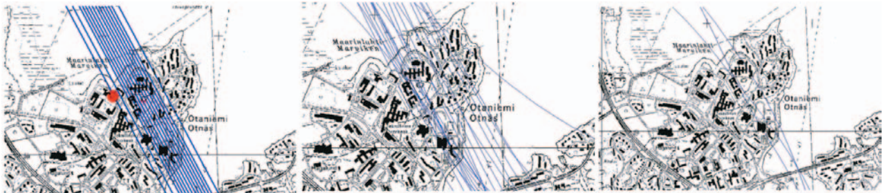
Figure A1-5. The planned and actual flight lines used in the Otaniemi 2000 exercise. The bigger red spot on the left is a big chimney. The source term is the smaller red line on that same picture. The three lines at the right were flown in opposite directions.
