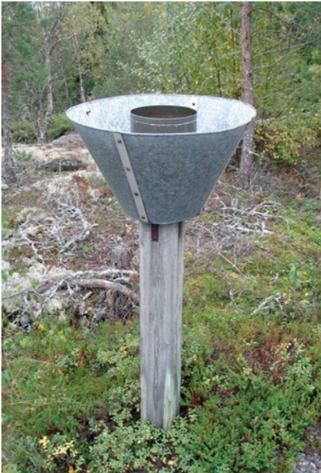
Fig. 3. The collector for tritium in rainwater.
