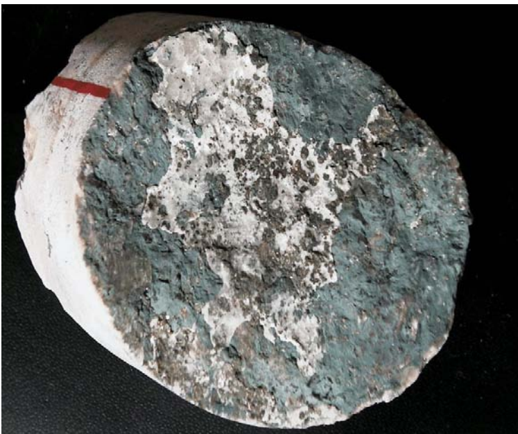
Figure 9. Typical clay filled fracture with a calcite coating that is partly covered by pyrite (from the core of OL-KR20 at 97.75 m depth). From Posiva (2009, p396).
