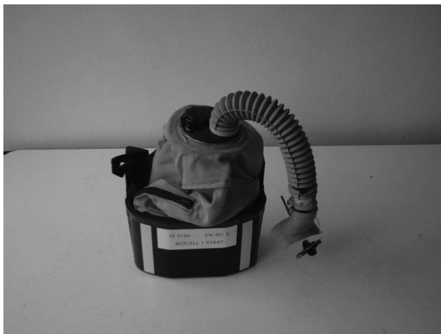
Figure 6. To enable the equipment for use, it is necessary to pull off the black plate on which the trachea is mounted. Usually, untrained individuals pull directly from the trachea, disabling the equipment.
