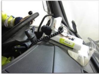
Picture 2. A digital infrared video camera for recording drivers at the wheel.
