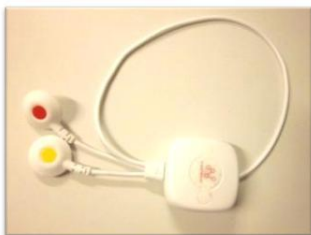
Picture 3. A heartbeat measurement device for recording heart rate variability.
