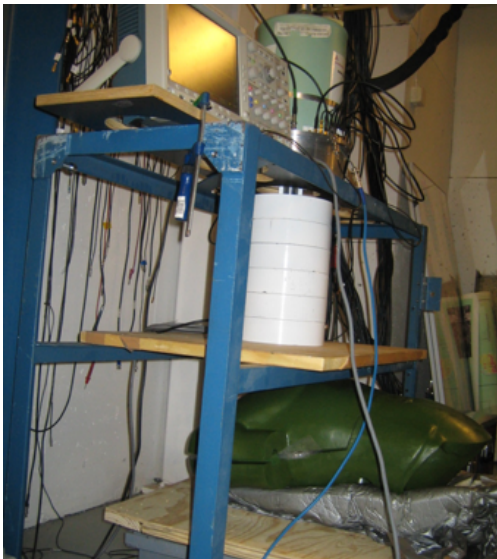
FIGURE 6. A large volume 36-fold segmented germanium detector mounted above a phantom used to investigate the methods to improve background suppression in full-body counting experiments.
