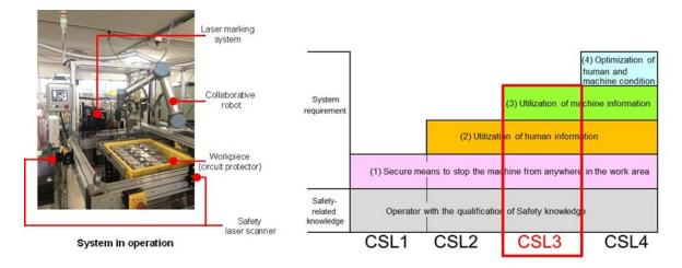
Fig. 2 Robot production system with Safety2.0-CSL3 (Cooperative safety level 3) using a collaborative robot
