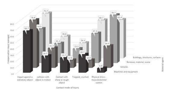
Figure 1: Compensated days on average against Contact mode of injuries and Material agent.
