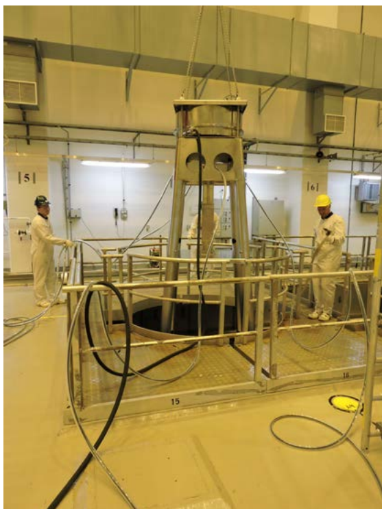
FIGURE 7. Setting up the measurement campaign with PGET and PNAR at Olkiluoto spent fuel storage, July 2019.
