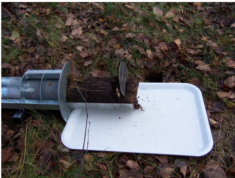
Figure 2. Slicing of a soil sample taken with a golf hole cutter. Photo: STUK.
