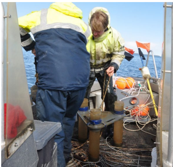
Figure 7. A collector of sinking matter. Photo: STUK.
