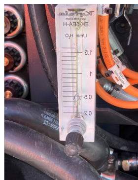
Figure 3 c. Water supply adjustment of drill rig (ca. 0,4 l/min)
